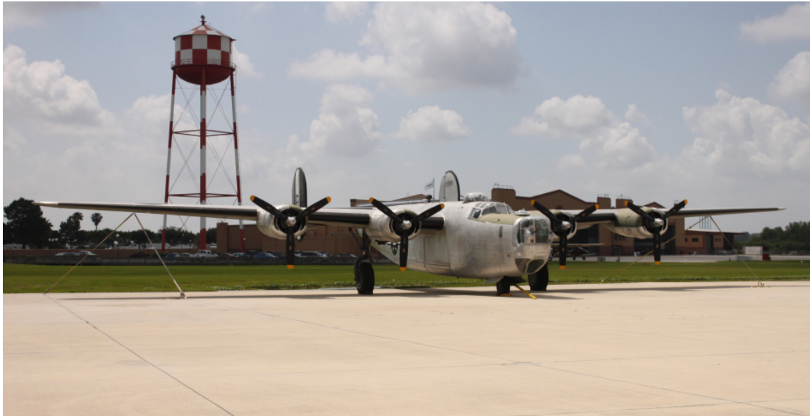
Figure C1-27: A Consolidated B-24J-90-CF Liberator (USAAF Code 44-44272) bomber built in 1944 parked in Polk City, Florida, boasting its high Aspect Ratio Davis wing. (Photo by Phil Rademacher)
