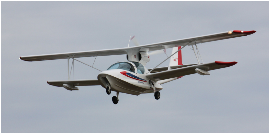
Figure C1-1: An EDRA Super Petrel LS on final. The airplane combines a number of configuration features presented in appendices C1 and C3; an amphibian, a biplane, and a pusher. (Photo by Phil Rademacher)
