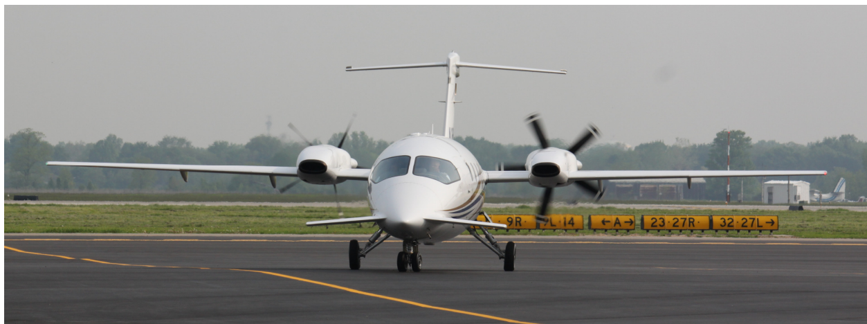
Figure C1-18: A Piaggio P.180 Avanti turboprop taxiing. The forewing features a flap that deploys when the main wing flaps are deployed to help counter the nose-down pitching moment. (Photo by Phil Rademacher)
